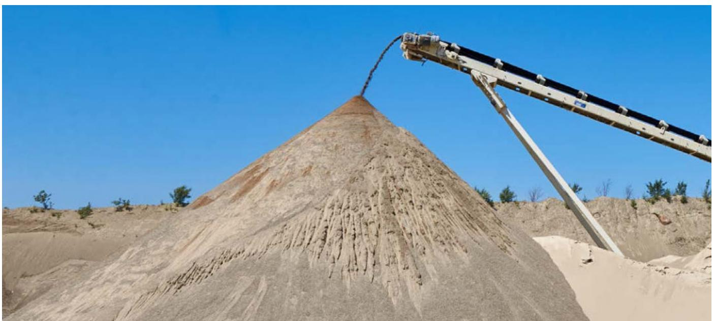
**Figure 4: Sand being manufactured from a stone quarry source**
