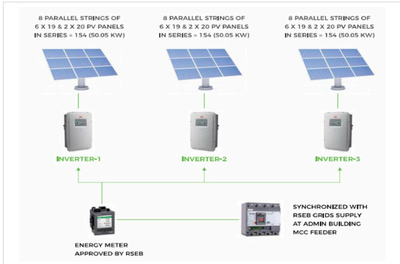
**Figure 5: Solar PV System arrangement**
