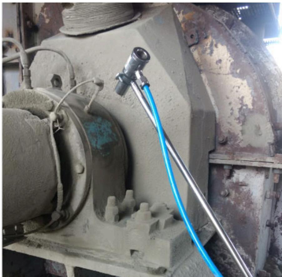
**Bearing housing cooling by Energy efficient device
